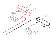
Place electrodes on the wrists. Register cardio signal for 5 minutes.
